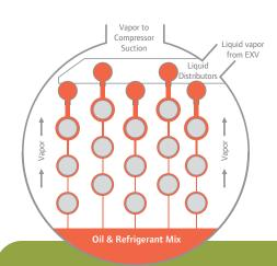
Our patented evaporator design gives the Trane RTWD higher efficiencies using less refrigerant charge, both of which contribute to LEED certification. Refrigerant (red) is uniformly distributed over the first row of tubes. It then flows around them, precisely at the points where heat transfer occurs, to more efficiently cool the fluid (blue) inside.
